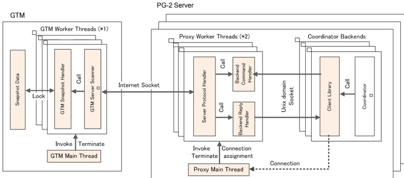
\*1 GTM Server Worker Thread is created when new connection from the proxy is accepted.
